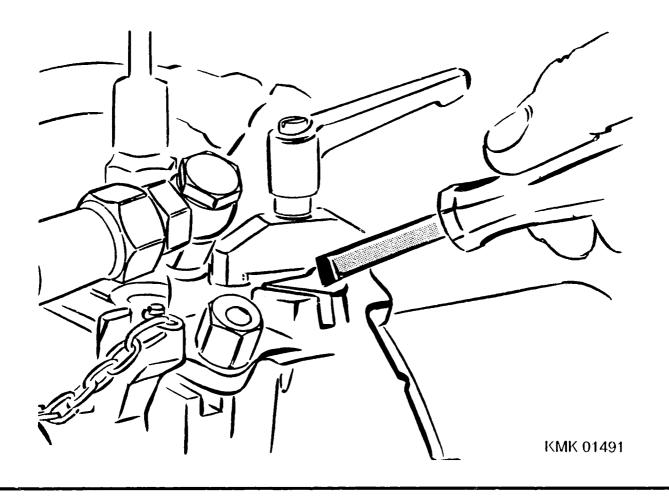
Move control rod to "0" position and set with setting mandrel of driving device.
